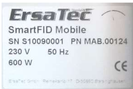
Figure 2: Identification plate SmartFID mobile
