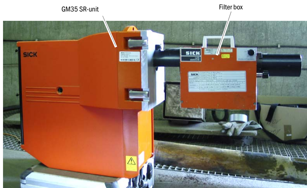
Fig. 73: Installing the filter box
