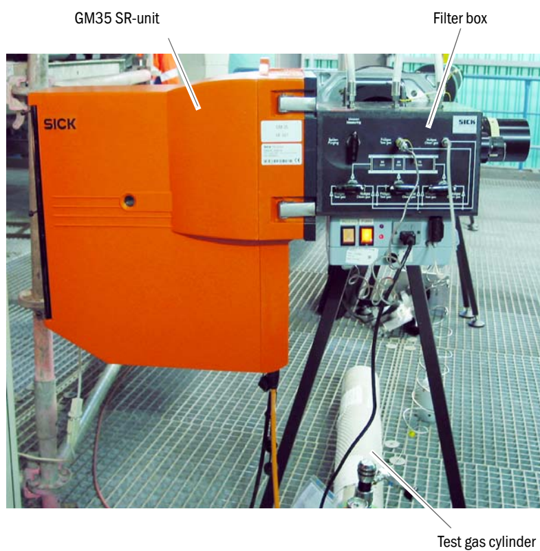
Fig. 71: Installing the filter box
