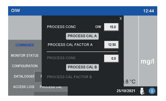
5. Press and hold PROCESS CAL A (or B depending on the probe you want to calibrate if more than one are present).
