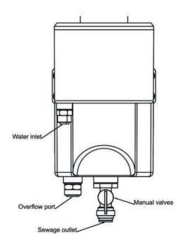
The sample reservoir (included with the purchase of the low range probe) should be mounted preferably under the controller. Connect the sample line to the water inlet on the left side. Then connect the outlet to drain. The manual drain outlet can be connected to drain or left free.
