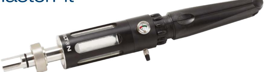
The MasterFit is a housing for pressurizable pH sensors like the ChemoTrode types. The pressurization ensures a constant outflow of electrolyte. This helps to prevent clogging of the diaphragm and poisoning of the electrolyte. The MasterFit can be used in a huge variety of applications mainly in the chemical industry.
