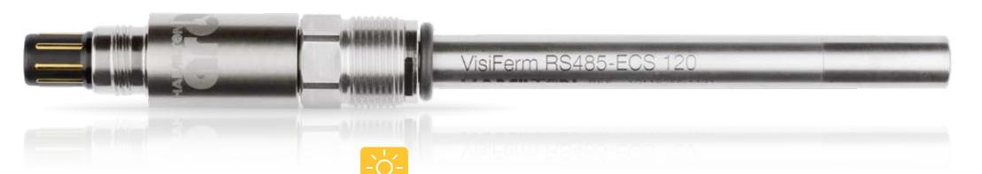
The VisiFerm RS485 is the first optical oxygen sensor with integrated opto-electronics, having the full functionality of a measuring device with self-diagnostics. It is steam sterilizable, autoclavable and CIP compatible. The VisiFerm requires less maintenance than a classical oxygen sensor as it does not have a mechanically sensitive membrane or a corrosive electrolyte.
