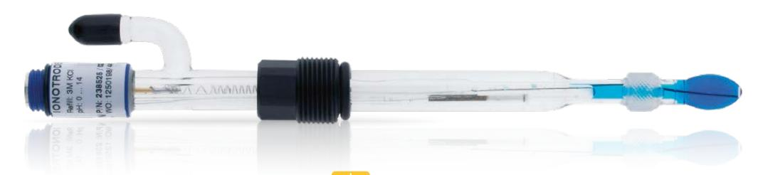
**Specifications** Measuring range 0 to 14 pH Process temperature -10 to 40 °C 0 to 0.5 bar or higher if Pressure range (relative to ambient) pressurization by side-arm pH glass 3 M KCI Electrolyte Reference system Everef Diaphragm Sleeve **EPDM** O-ring
