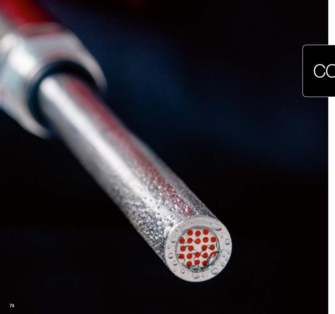
Dissolved carbon dioxide (DCO<sub>2</sub>) is a critical process parameter (CPP) in biopharma production processes according to PAT guidelines. By influencing other parameters such as extracellular and intracellular pH, it has an effect on different metabolic pathways which are involved in cell growth or in product formation and quality.
