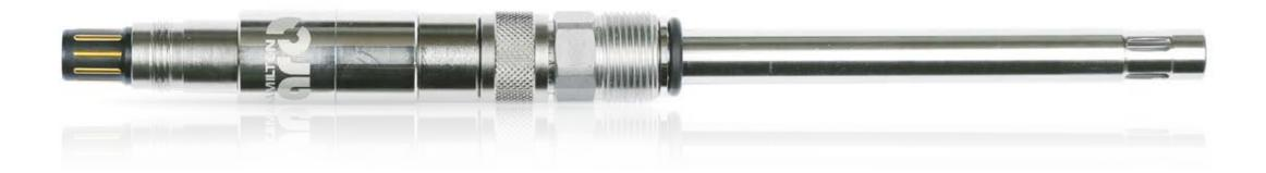
**Specifications** Measuring range 0.01 to 1500 µS/cm Measurement Principle 2 pole contacting Arc: analog 0 to 110 °C, Process temperature digital 0 to 130 °C Pressure range 0 to 10 bar (130 °C) (relative to ambient) Autoclavable, CIP, SIP Hygienic aspects Cell constant < 0.1/cmMaterial of electrodes Stainless Steel DIN 1.4435 Surface quality  $R_a < 0.4 \ \mu m \ (N5)$ O-ring EPDM (other versions available on request)
