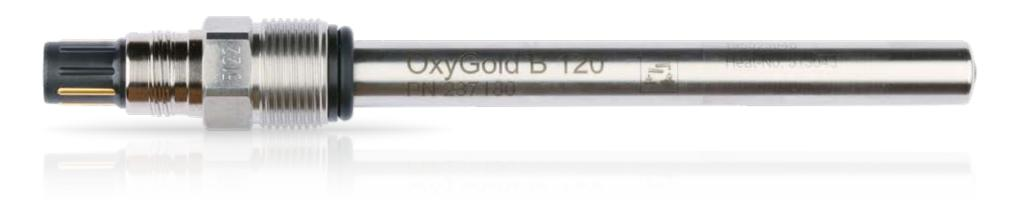
**Specifications** Measuring range 8 ppb to 40 ppm (DO) Response time t98% < 60 s at 25 °C, from air to nitrogen 0 to 100 °C Process temperature Pressure range 0 to 12 bar (relative to ambient) CIP Hygienic aspects Oxylyte B Electrolyte Surface Quality  $R_a < 0.4 \mu m (N5)$ Current in air at 25°C 180 to 500 nA Material Stainless steel 1.4435 Polarization voltage 0 mV **EPDM** O-ring
