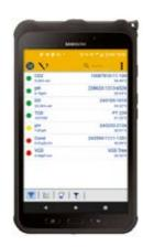
This mobile device empowers the operator to monitor measurement values, calibrate Arc sensors and configure various parameters with a unified user interface for pH, DO, Conductivity and ORP. The Arc View Mobile device is based on the Samsung Galaxy Tab Active tablet and comes pre-configured with the ArcAir application, app blocker application and power supply.
