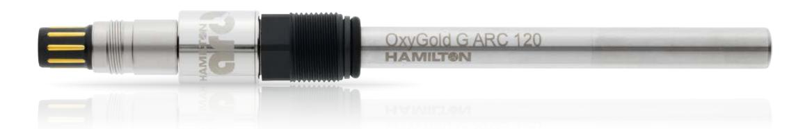
**Specifications** Measuring range 1 ppb to 40 ppm (DO) Response time t98% < 60 s at 25 °C, from air to nitrogen Process temperature 0 to 130 °C (Arc: analog 0 to 110 °C, digital 0 to 130 °C) Pressure range 0 to 12 bar (relative to ambient) Hygienic aspects Autoclavable, CIP, SIP Electrolyte Oxylyte G Surface Quality  $R_a < 0.4 \mu m (N5)$ Current in air at 25°C 180 to 500 nA Stainless steel 1.4435 Material -670 mV Polarization voltage **EPDM** O-ring
