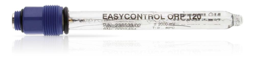
**Specifications** Measuring range  $\pm$  2000 mV Process temperature 0 to 60 °C 0 to 2 bar Pressure range (relative to ambient) ORP element Pt-wire Electrolyte Gel electrolyte Ag/AgCI Reference system Diaphragm Ceramic **EPDM** O-ring
