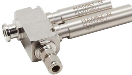
Hamilton Flow-Through Cells are designed for measuring one or two parameters at a time. Possible combinations are pH/DO and pH/Conductivity. The measurement is done in bypasses when inline measurement is not possible due to small pipe dimensions. Application fields are biotechnology, water treatment and power plants, where reliable measurements have to be carried out in ion-weak media. There are two different sizes of the flow cells available.
