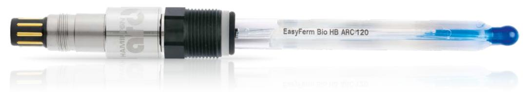
**Specifications** Measuring range 0 to 14 pH Process temperature 0 to 140 °C (Arc: analog 0 to 110 °C, digital 0 to 140 °C) 0 to 6 bar Pressure range (relative to ambient) Hygienic aspects Autoclavable, SIP, CIP HB, PHI pH glass Electrolyte Foodlyte Reference system Everef-F Diaphragm **HP** Coatramic O-ring Silicone
