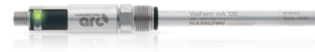
**Specifications** 4 ppb to 25 ppm (DO) Measuring range Measurement Principle Oxygen dependent luminescence quenching Response time t98% < 30 s at 25 °C, from air to nitrogen Process temperature -20 to 140 °C, the sensor provides no DO reading above 85 °C Operating voltage 18 to 30 VDC Pressure range -1 to 12 bar (relative to ambient) Hygienic aspects Autoclavable, CIP, SIP Surface Quality  $R_a < 0.4 \mu m (N5)$ Stainless steel 1.4435 Material O-ring **EPDM**
