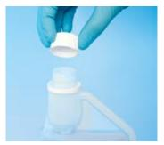
Step 2 Fill calibration compartment
