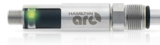
**Specifications** 0 to 2000 ppb (DO) Measuring range Measurement Principle Oxygen dependent luminescence quenching Response time t<sub>98%</sub> < 20 s in gas; < 90 s in water Process temperature -20 to 140 °C, the sensor provides no DO reading above 85 °C Operating voltage 18 to 30 VDC Pressure range -1 to 12 bar (relative to ambient) Hygienic aspects Autoclavable, CIP, SIP Surface Quality  $R_a < 0.4 \mu m (N5)$ Material Stainless steel 1.4435 O-ring **EPDM**
