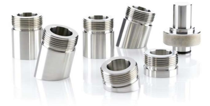
The Safety Sockets are hygienic weld-in sockets suitable for hygienic armatures like the FlexiFit Bio. They are available for 3 different o-ring positions to cover different standards. Furthermore you can choose between two kinds of stainless steel and two different angles.
