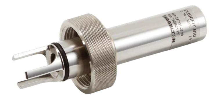
The FlexiFit housings are designed for 120 mm sensors in different kinds of industries. A variety of process connections ensure the usability in the chemical industry as well as in hygienic processes. All FlexiFit have EPDM o-rings and the electropolished surface quality (Ra < 0.4  $\mu$ m) quality is shown on a certificate. They are suitable for autoclavation, CIP and SIP procedures.
