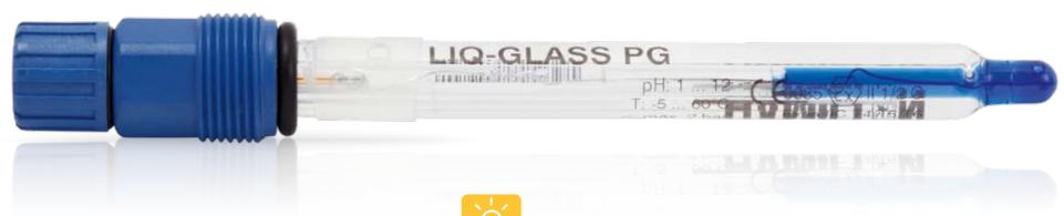
The maintenance free Liq-Glass PG and the EasyControl sensors are entry level sensors for chemical or waste water applications and low process temperatures. They show good behaviour in samples with low conductivity.
