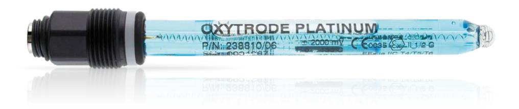
**Specifications** Measuring range ± 2000 mV 0 to 130 °C Process temperature 0 to 16 bar (25 °C) Pressure range 0 to 6 bar (130 °C) (relative to ambient) ORP element Pt wire Viscous 3 M KCI-Pharma, blue Electrolyte Reference system Everef HP ceramic Diaphragm **EPDM** O-ring
