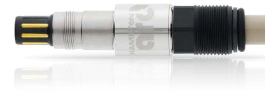
**Specifications** 1  $\mu$ S/cm to 300 mS/cm Measuring range Measurement Principle 4 pole contacting Process temperature -20 to 150 °C (Arc: analog 0 to 110 °C, digital 0 to 140 °C) 0 to 20 bar (135 °C) Pressure range (relative to ambient) 0 to 10 bar (150 °C) Autoclavable, CIP, SIP Hygienic aspects Cell constant 0.36/cm Material of electrodes S = Stainless steel 1.4435 H = Hastelloy C 2.4602 T = TitaniumPt = Platinum O-ring EPDM (other versions available on request)
