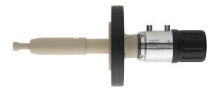
The retractable pneumatic armature Retractex C Plastic LT M was designed for harsh applications in the chemical industry. The compact design with a stroke of only 36 mm with an insertion depth of 194 mm keeps wear on seals to a minimum and creates excellent reliability. It can be cleaned easily and thoroughly in place. It is designed for 12 mm sensors and is equipped with several safety features (e.g. no sensor – no insertion, window to check seals for leakage etc.) to provide operator safety.
