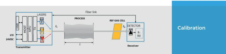
Each GasEye<sup>™</sup> analyzer is equipped as standard with auto-calibration features for real-time monitoring of system status. The reference signal from a reference gas always present is the measurement path ensures correct measurement even in the most demanding conditions. This feature removes the necessity to perform calibration on-site and keeps your overall maintenance effort low. Proven-in-use: verified in several million operating hours with failure rates fulfilling SIL2.
