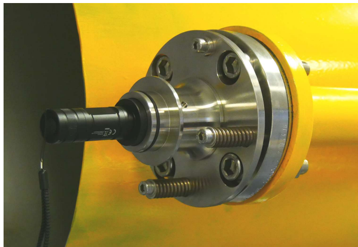
Figure 24. Placing the light source.
